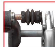
**APPEARANCE** Uneven wear of brake pads on one brake caliper
