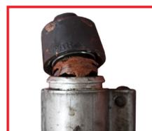
**APPEARANCE** Rust around brake cylinder pins
