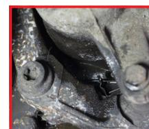
**APPEARANCE** Rust around brake caliper piston
