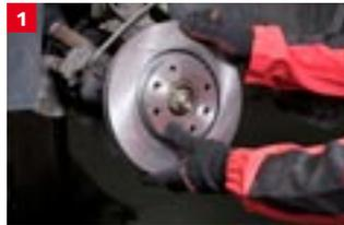
**DESCRIPTION** A deep noise with frequency below 300 Hz. It normally originates from macro-vibrations of a brake system component e.g. the disc
