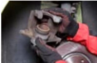
> Check for free piston movement, and retract the piston fully – this is essential to avoid damage to the shim or the rubber coat.
