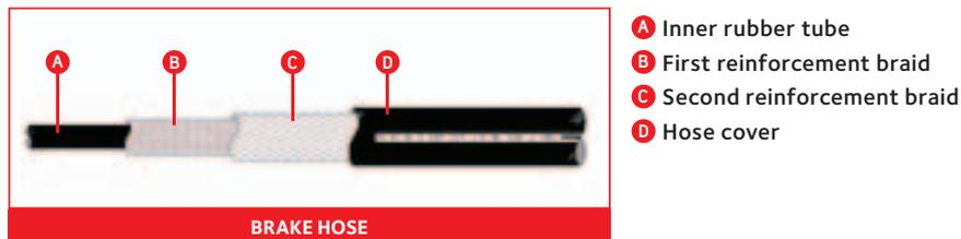
The aging process can act differently on different parts of the hose.
