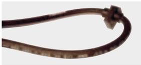
> Contact of the exterior of the hose with fluid, mineral oil or grease
