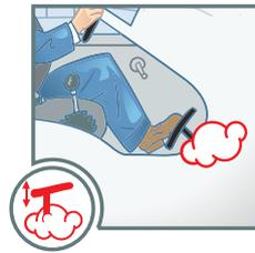
Spongy pedal feel is the experience where upon depressing the brake pedal, the brake is slow to respond, and the pedal feels spongy – softer than it should be, with excessive force required to decelerate the vehicle and excessive stroke of the pedal.
